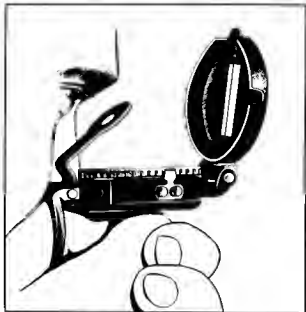
Figure 35. A method of holding the compass.
